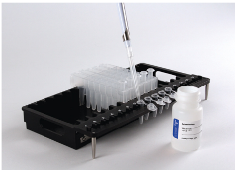
Figure 2. Setup and configuration of the deck tray(s). Elution Buffer is added to the elution tubes as indicated. Deck tray shown is from the Maxwell ® RSC Instrument (Cat.# AS4500).
