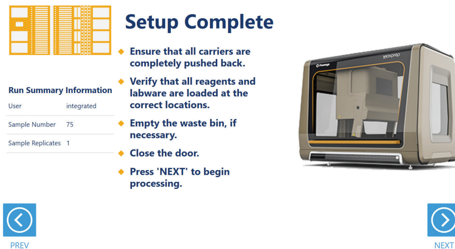
Figure 20. Final instrument setup screen. This screen presents a list of items that should be checked before starting automated processing. It also provides a final chance to return to any of the previous instrument setup screens before automated processing begins. To start processing, close the instrument door and press the Next button.
