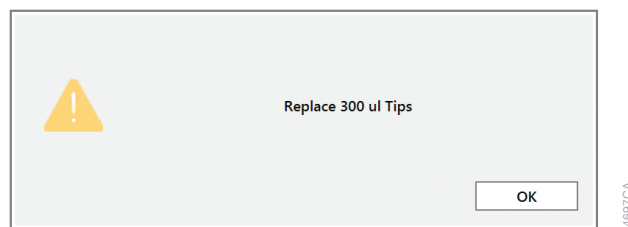
Figure 22. Insufficient tips on the system to complete a method. In the event that all tips of a given tip type are consumed during a run, the instrument will pause and unlock the door. Open the door, load more tips of the indicated type on the tip and plate carrier, close the door and press OK to resume processing.
